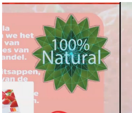
Figure 2. Implementation of the Smart Select function when the program analyzes the context of the image and correctly selects the logo without capturing the surrounding background.
